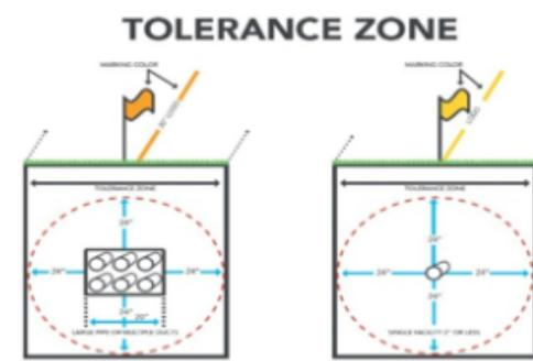
Employ hand tools or other non-invasive methods either to determine the exact location of the underground facility or down to 24 inches beyond the depth of intended excavation within 24 inches of the outside dimensions of a marked underground facility.
